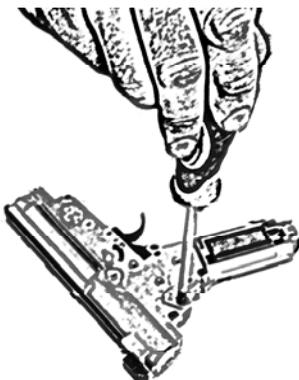
Remove the transmitting semi-gearwheel and the engine bed with the motor.
