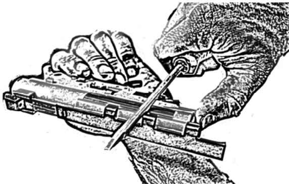
Remove the halves connecting strip from the gearbox.
